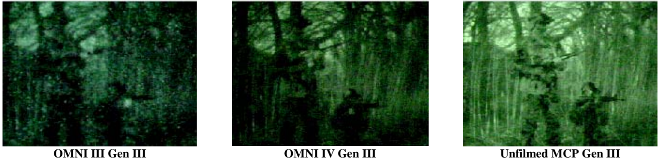
Fig. 10. Ground Field Comparison of I 2 Technologies ( 2 \times 10^{-5} fc light level)
