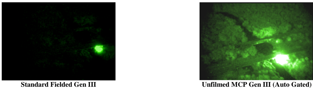
Fig. 11. Aerial Comparison of Autogated Unfilmed Gen III I 2 to Standard Gen III I 2
